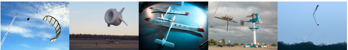
Fig. 1. Examples of Airborne Wind Energy generators. From left: a ground-based generator with soft kite from TU Delft [5], a buoyant system from Altaeros Energies [6], two rigid wings for ground-based generation by Ampyx Power [7], a 600-kW system with onboard generation from Makani Power-GoogleX [8], and a semi-rigid wing concept from EnerKite [9].
